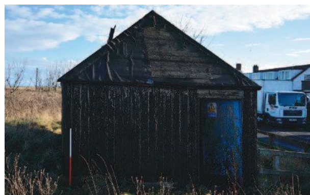
The remains of the fisherman's hut at Beadnell in Northumberland which was made and repaired using boat materials
