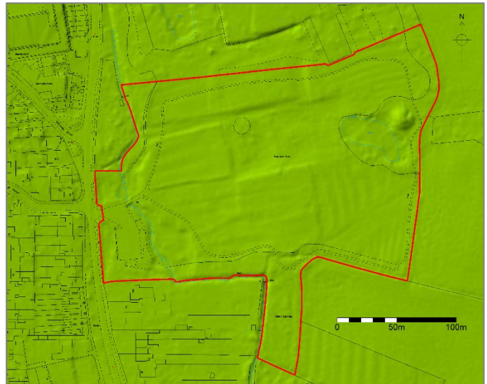
Above: This is a digital terrain model of the park generated using LiDAR, an airborne survey method which uses a laser to map the ground surface. The image has been processed to remove buildings and vegetation and reveal the shape of the ground beneath. The resulting model clearly shows the many earthworks in the park. Image: ULAS / Environment Agency / Ordnance Survey.
